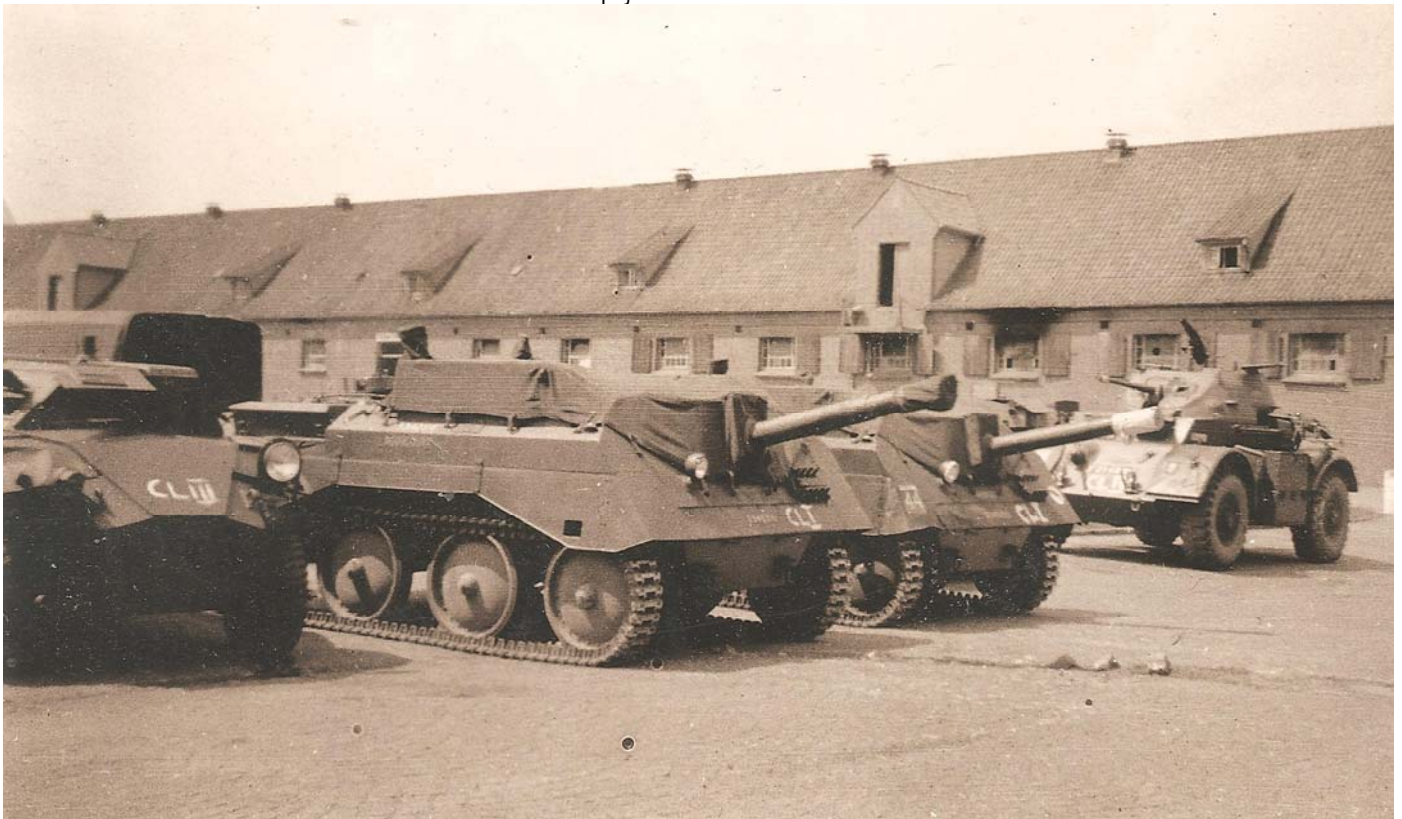
Image courtesy of the Trooper Alfred William Bolden who served between 1942-1947. Description: Having had the turrets removed to be fitted onto the Daimler heavy armoured car, these Tetrarch light tanks were reconfigured to accommodate a heavy gun and were designated Electra's. This photo at the end of the war shows them lined up for disposal, The Humber scout car is Class III (poor condition and probably destined for scrapping), and the electras both Class I (good condition).
